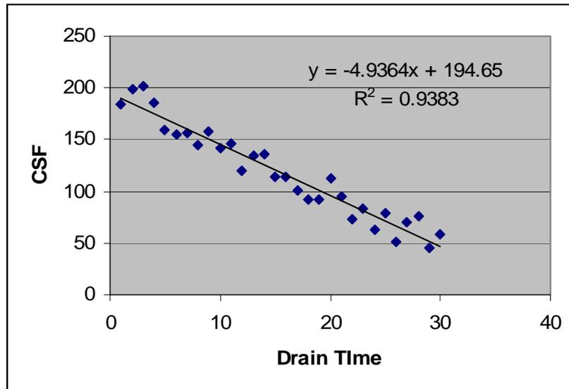
Figure 2: Drain Time and Lab Evaluations of Freeness
