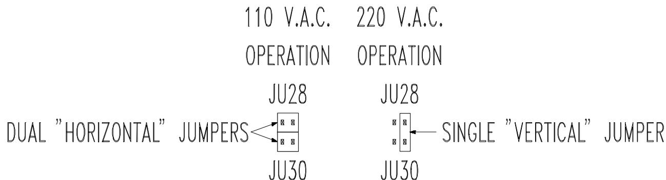
Figure 6 Operating Voltage Jumpers
