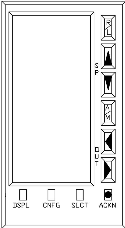
Figure 28 Operator Keys
