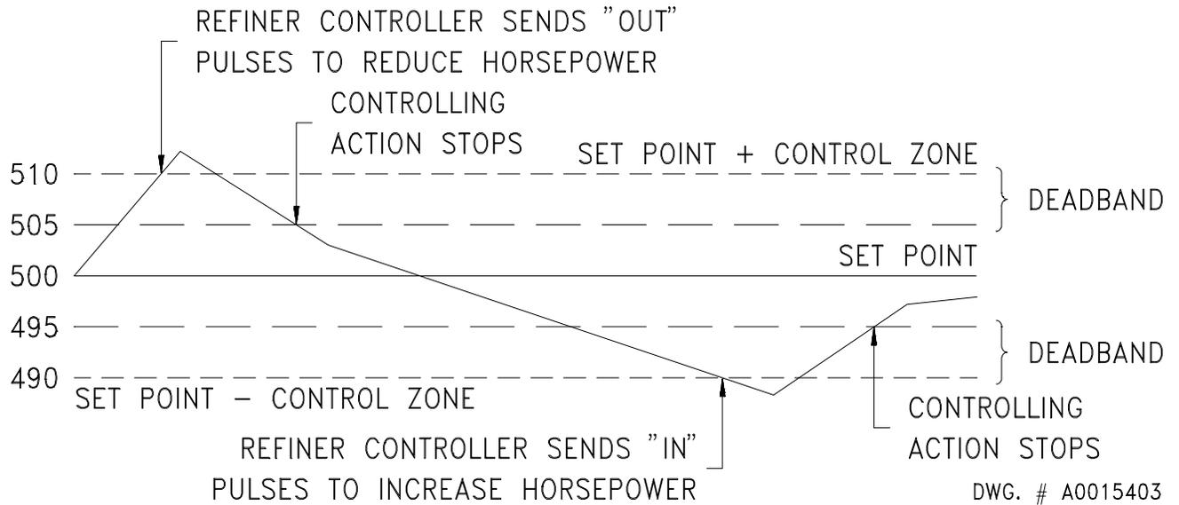
Figure 9 Control Zone, Deadband And Controller Action
