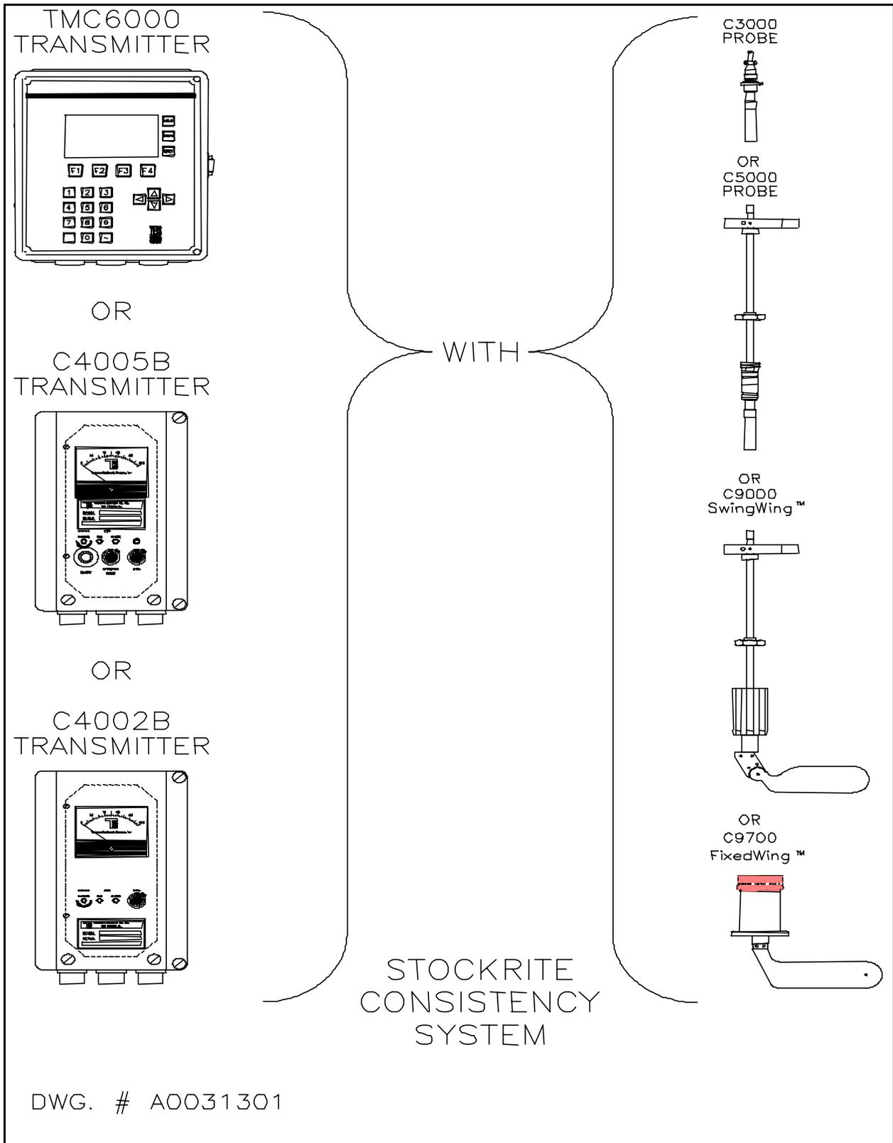
**Figure 1** Stockrite™ Consistency System
