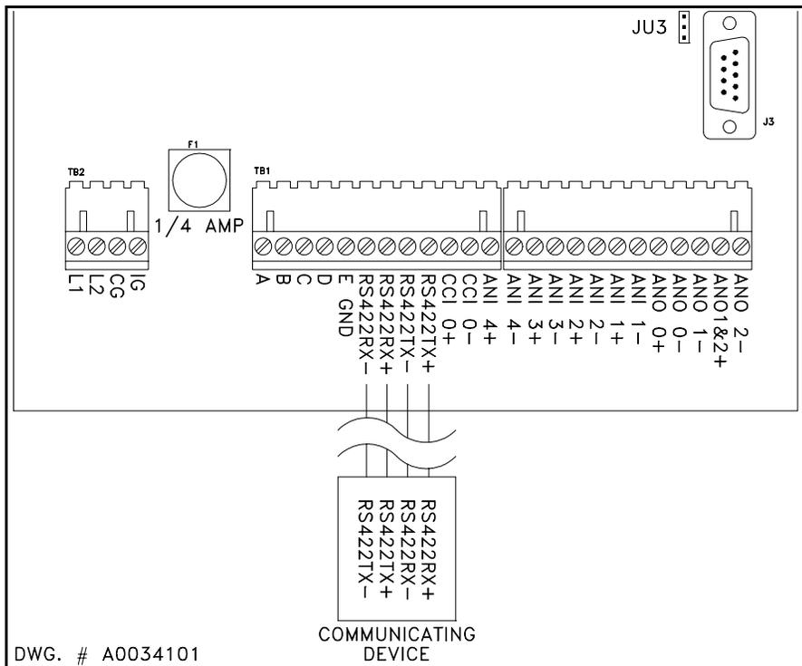
**Figure 26** RS422/485 Wiring Configuration
