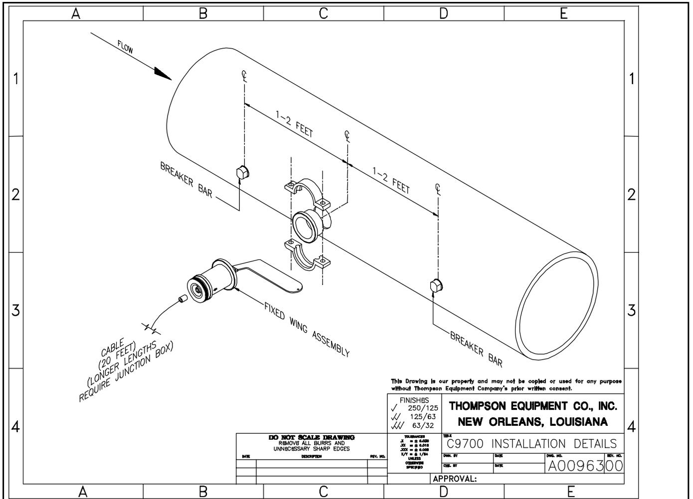
Figure 20 C9700 FixedWing™ Installation
