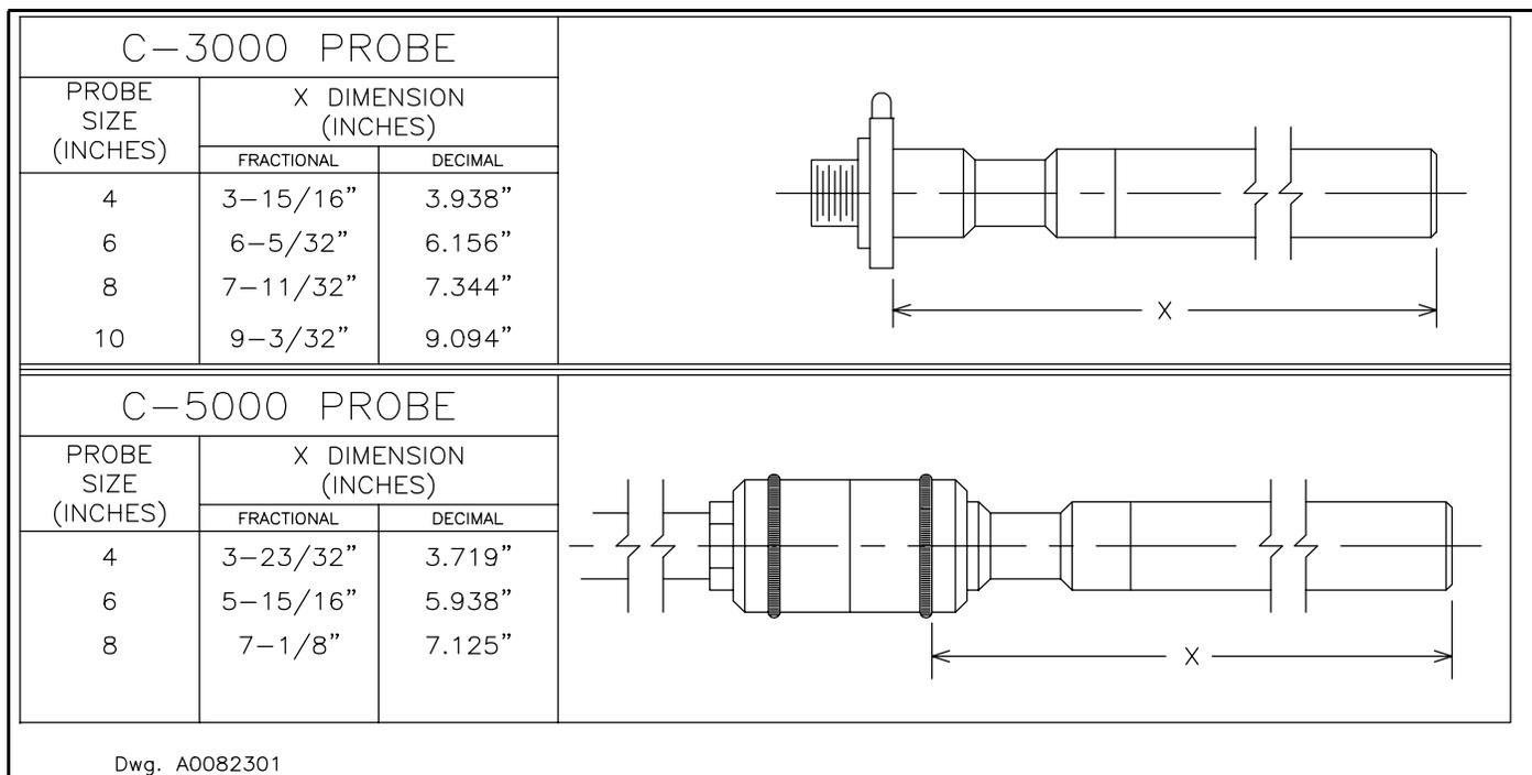
**Figure 15** Probe Identification
