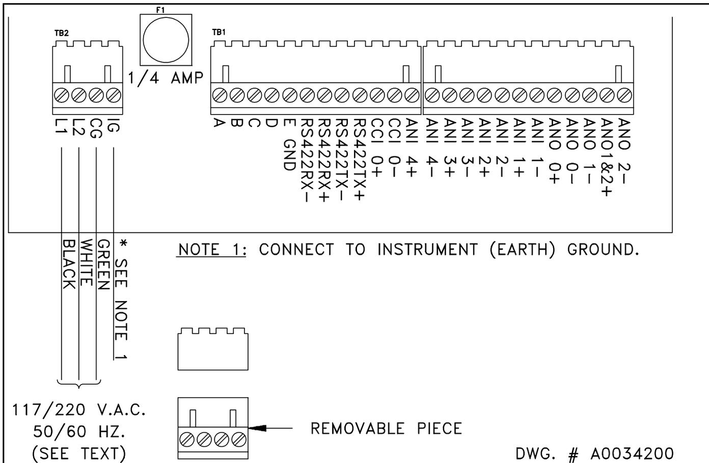
**Figure 8** Power Wiring Connections
