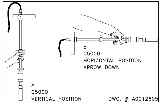
Figure 3 C5000 Calibration Positions
