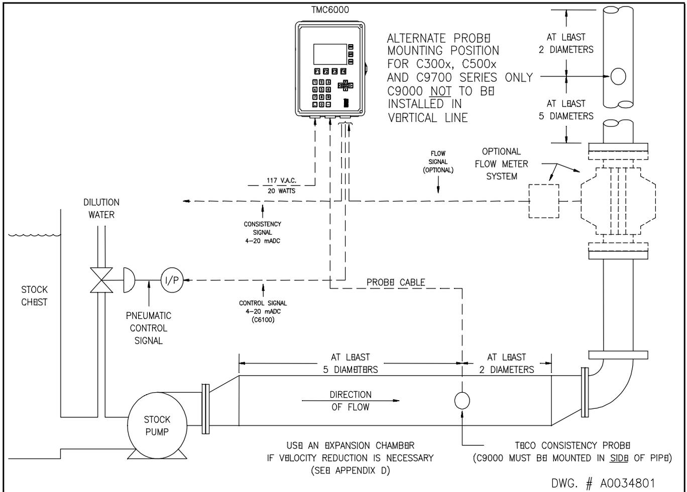
**Figure 6** TECO Stockrite™ Consistency System Installation
