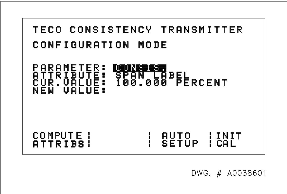
**Figure 34** Configuration Display
