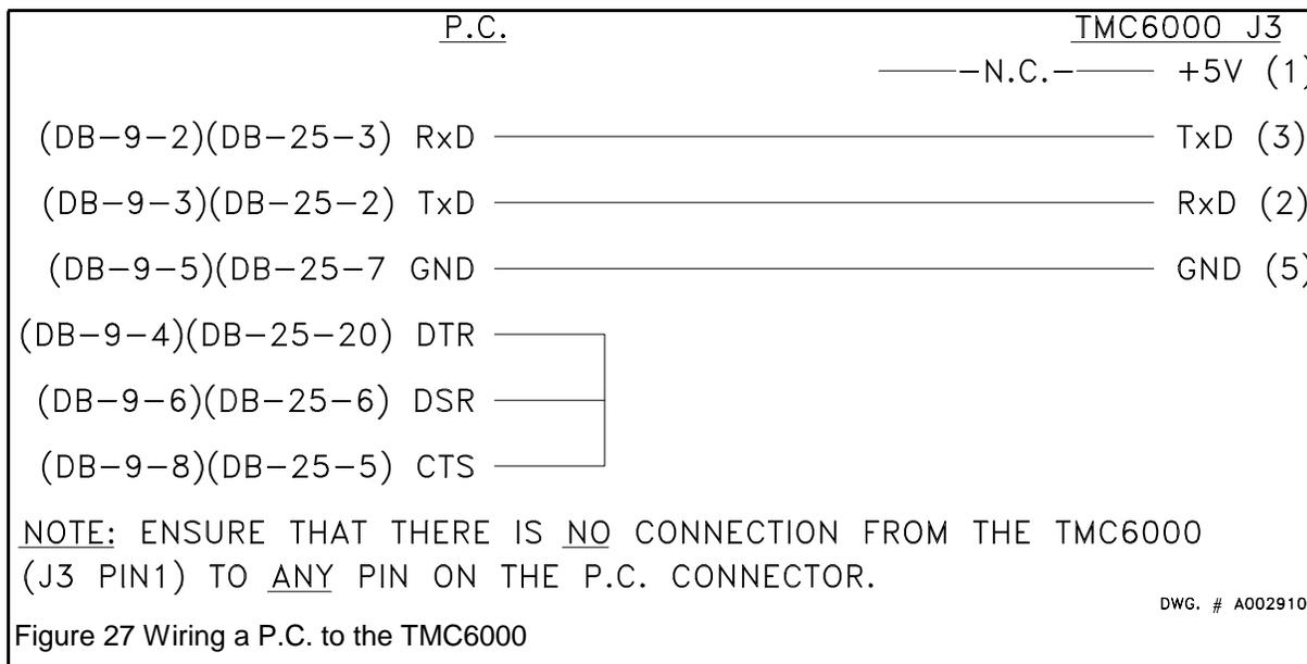
**Note:** The TMC6000 J3 Pin 1 does NOT conform to standard RS-232 signal definition. It is used to provide power for a hand-held configurer and MUST NOT be connected to ANY pin in a P.C. Damage to either the TMC6000 serial interface or the P.C. serial interface may occur.
