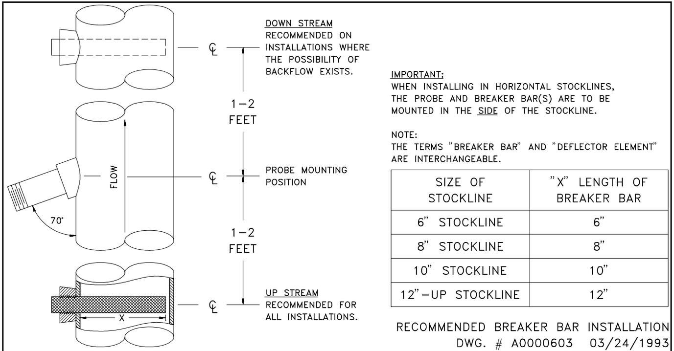
**Figure 14** Breaker Bar Installation
