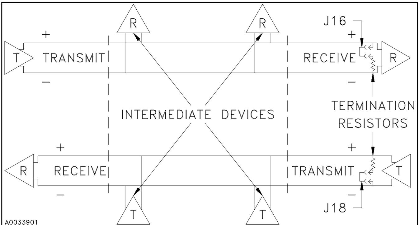
Figure 24 RS422/485 Communication Block Diagram
