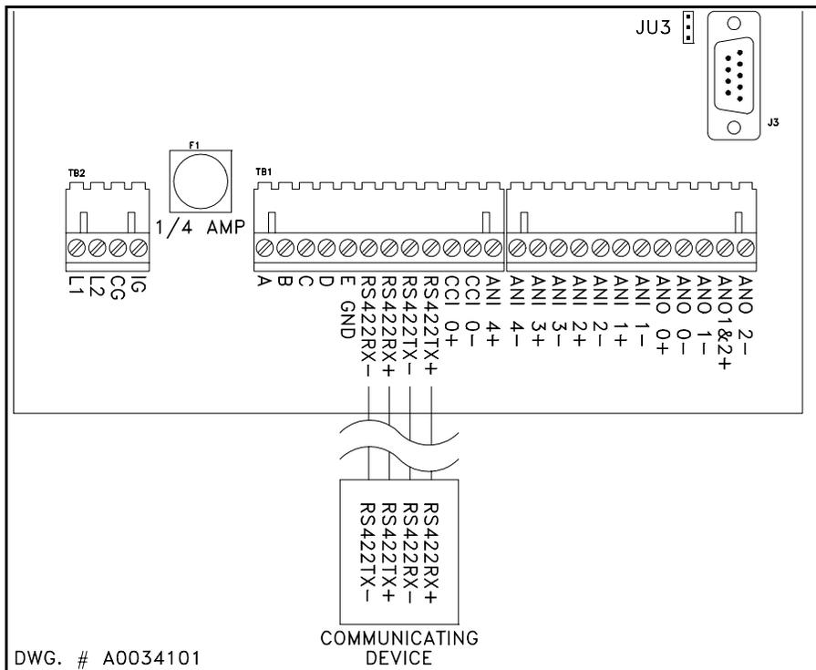
**Figure 26** RS422/485 Wiring Configuration
