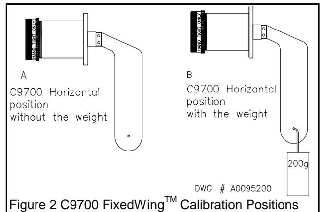
Figure 2 C9700 FixedWing™ Calibration Positions
