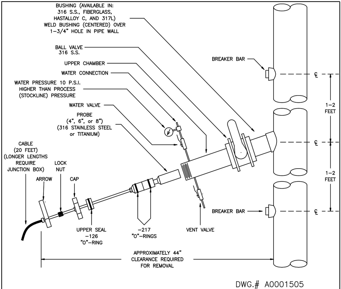
Figure 17 C5000 Removable Probe Installation
