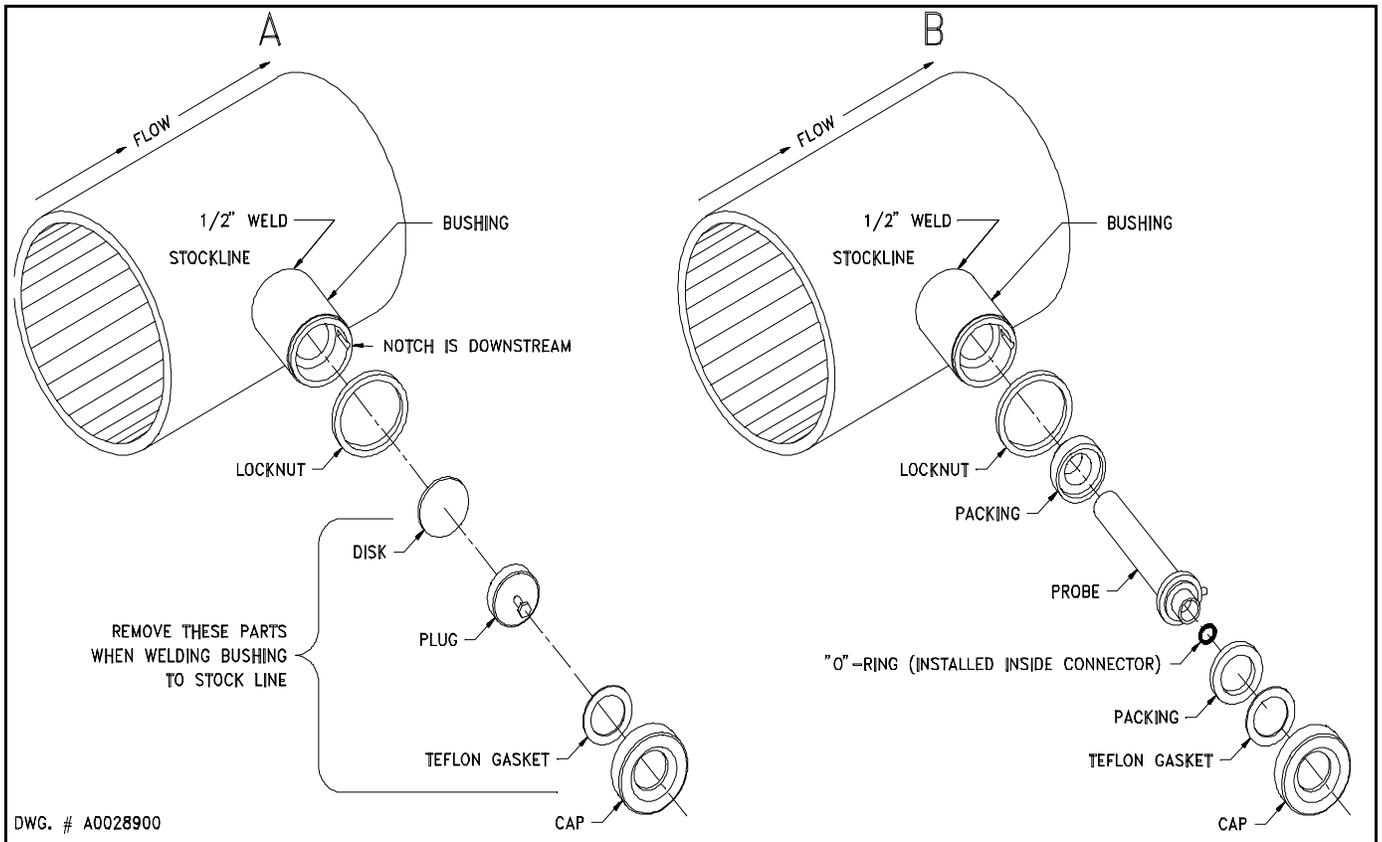
**Figure 16 C-3000 Bushing & Probe Installation**
