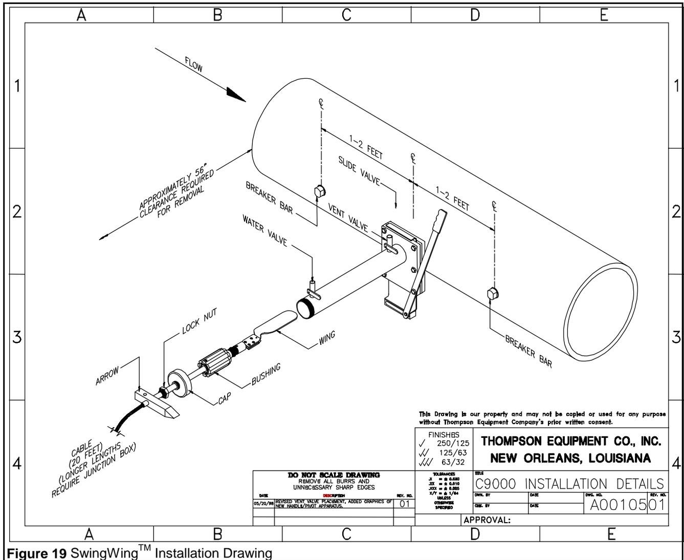
Figure 19 SwingWing™ Installation Drawing
