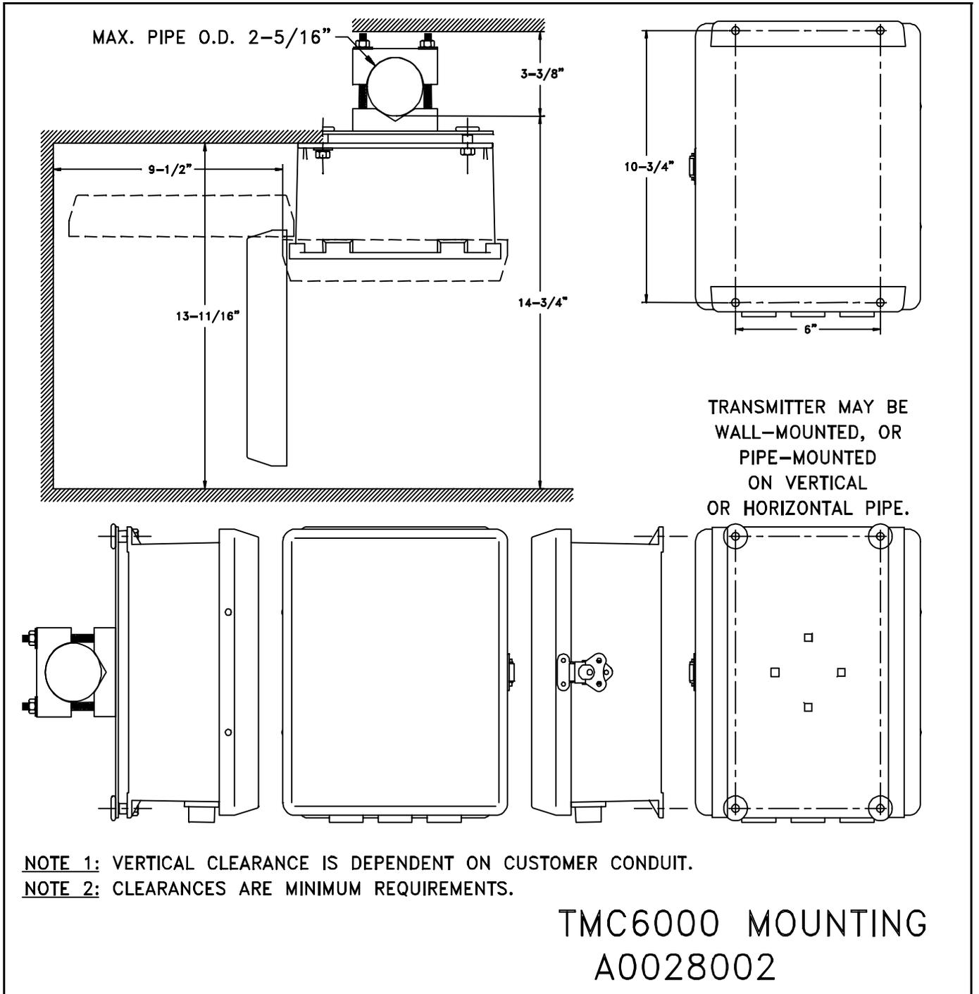
**Figure 7** Transmitter Mounting Dimensions
