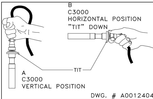
Figure 4 C3000 Calibration Positions
