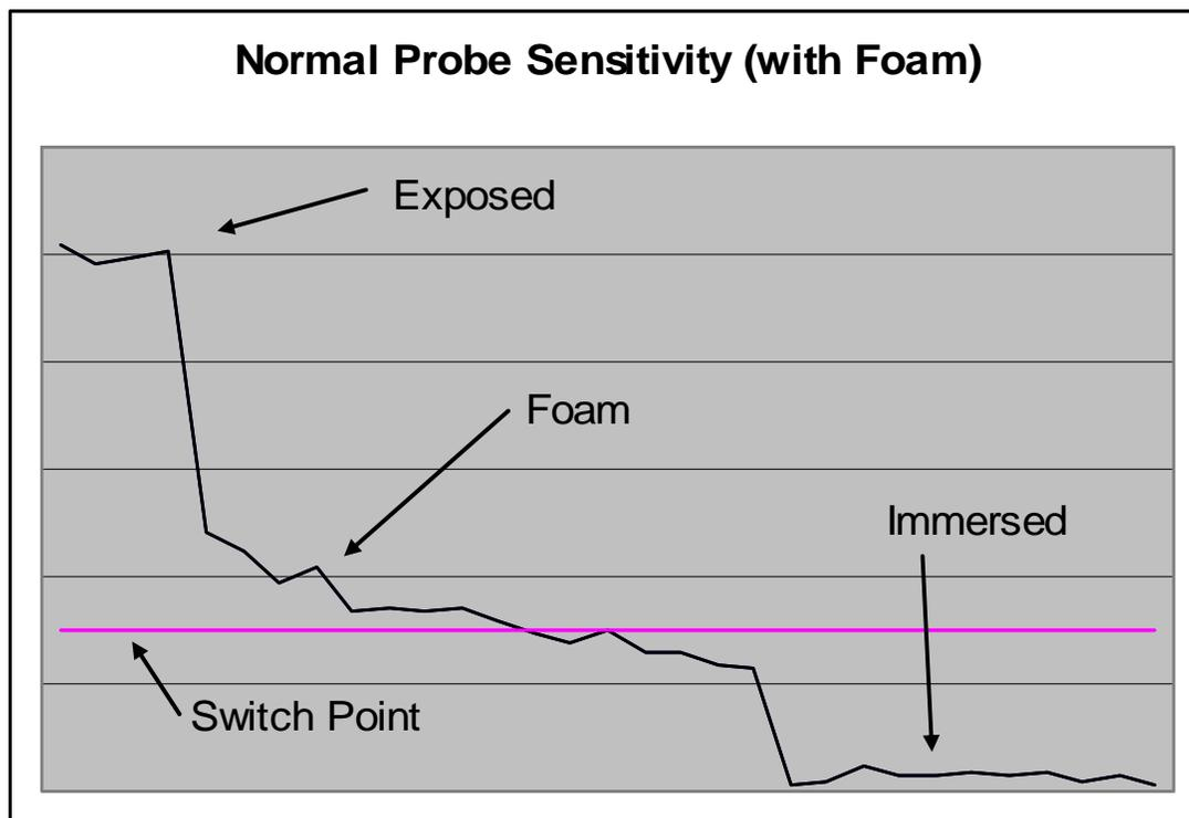
Figures 4: Probe Resistance with Normal  $P_{sen}$  and Foam
