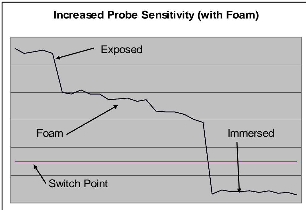
Figure 5: Probe Resistance with Increased Probe Sensitivity Setting
