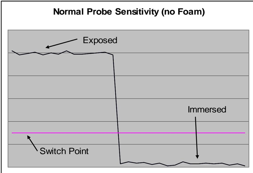
Figure 3: Probe Resistance with Normal  $P_{sen}$  and no Foam Present
