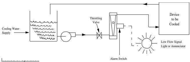
The required amount of cooling water is easily set and monitored by the use of a Rotameter. If the heat load varies, resetting the cooling water flow is easily accomplished due to the inherently easy readability of the Rotameter scale. A low flow alarm switch set at a slightly lower than the normal flow rate gives an immediate warning of a decreasing total interruption of flow.
