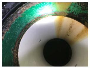
This TECO SAM had 500,000,000 pounds of sand flow through its core. Upon inspection, the customer found the flow tube to be looking "brand new". The unit was put back in service and has exceeded 2,000,000,000 pounds of sand and <u>has yet to fail</u>.
